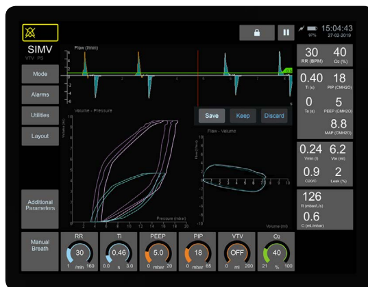
Loops A lung mechanics screen shows additional data - in this case two loops. A secondary column of data can be shown when required.
