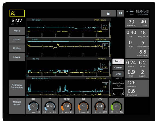
Trends Up to 14 days of trends are stored for all parameters. Zoom and scroll to find any parameter's values at a particular time.
